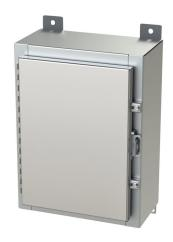
Saginaw enclosure, NEMA 3R/4/4X/12/13, 16 x 12 x 6in (HxWxD), wall mount, 304 stainless steel, #4 brush finish, single-door, stainless steel clamps, padlock hasp and staple.
