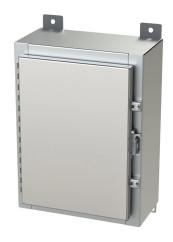
Saginaw enclosure, NEMA 3R/4/4X/12/13, 16 x 12 x 6in (HxWxD), wall mount, 316L stainless steel, #4 brush finish, single-door, stainless steel clamps, padlock hasp and staple.
