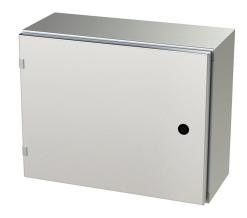
Saginaw Enviroline series enclosure, NEMA 3R/4/4X/12/13,  $16 \times 20 \times 8$  in (HxWxD), wall mount, 316L stainless steel, #4 brush finish, single-door, 1/4-turn semi-flush latch.
