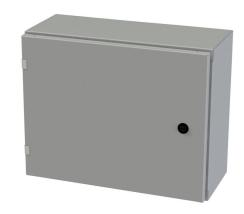
Saginaw Enviroline series enclosure, NEMA 3R/4/12/13,  $16 \times 20 \times 8$  in (HxWxD), wall mount, carbon steel, ANSI 61 gray, powder coat finish, single-door, 1/4-turn semi-flush latch.
