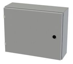
Saginaw Enviroline series enclosure, NEMA 3R/4/12/13,  $16 \times 20 \times 6in$  (HxWxD), wall mount, carbon steel, ANSI 61 gray, powder coat finish, single-door, 1/4-turn semi-flush latch.
