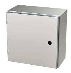
Saginaw Enviroline series enclosure, NEMA 3R/4/4X/12/13,  $16 \times 16 \times 8$  in (HxWxD), wall mount, 316L stainless steel, #4 brush finish, single-door, 1/4-turn semi-flush latch.
