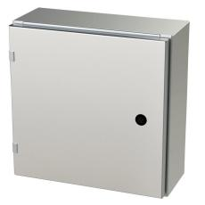
Saginaw Enviroline series enclosure, NEMA 3R/4/4X/12/13, 16 x 16 x 6in (HxWxD), wall mount, 316L stainless steel, #4 brush finish, single-door, 1/4-turn semi-flush latch.
