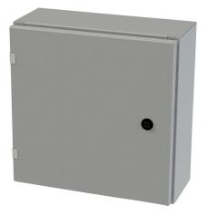
Saginaw Enviroline series enclosure, NEMA 3R/4/12/13,  $16 \times 16 \times 6$  in (HxWxD), wall mount, carbon steel, ANSI 61 gray, powder coat finish, single-door, 1/4-turn semi-flush latch.
