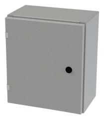
Saginaw Enviroline series enclosure, NEMA 3R/4/12/13,  $16 \times 14 \times 8in$  (HxWxD), wall mount, carbon steel, ANSI 61 gray, powder coat finish, single-door, 1/4-turn semi-flush latch.
