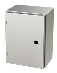
Saginaw Enviroline series enclosure, NEMA 3R/4/4X/12/13, 16 x 12 x 8in (HxWxD), wall mount, 316L stainless steel, #4 brush finish, single-door, 1/4-turn semi-flush latch.
