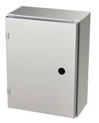
Saginaw Enviroline series enclosure, NEMA 3R/4/4X/12/13, 16 x 12 x 6in (HxWxD), wall mount, 304 stainless steel, #4 brush finish, single-door, 1/4-turn semi-flush latch.
