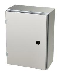
Saginaw Enviroline series enclosure, NEMA 3R/4/4X/12/13,  $16 \times 12 \times 6$  in (HxWxD), wall mount, 316L stainless steel, #4 brush finish, single-door, 1/4-turn semi-flush latch.
