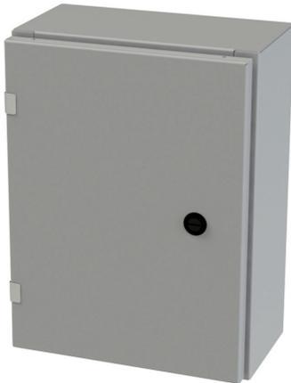
Saginaw Enviroline series enclosure, NEMA 3R/4/12/13, 16 x 12 x 6in (HxWxD), wall mount, carbon steel, ANSI 61 gray, powder coat finish, single-door, 1/4-turn semi-flush latch.
