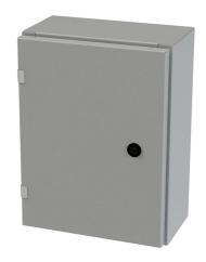
Saginaw Enviroline series enclosure, NEMA 3R/4/12/13,  $16 \times 12 \times 6$  in (HxWxD), wall mount, carbon steel, ANSI 61 gray, powder coat finish, single-door, 1/4-turn semi-flush latch.
