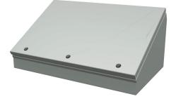
Saginaw operator consolet, NEMA 3R/4/12/13, 16 x 24 x 11in (HxWxD), desktop or pedestal mount, carbon steel, ANSI 61 gray, powder coat finish, single-door, 1/4-turn semi-flush latch.
