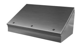
Saginaw operator consolet, NEMA 3R/4/4X/12/13, 16 x 24 x 11in (HxWxD), desktop or pedestal mount, 304 stainless steel, #4 brush finish, single-door, 1/4-turn semi-flush latch.
