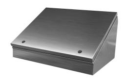
Saginaw operator consolet, NEMA 3R/4/4X/12/13, 16 x 20 x 11in (HxWxD), desktop or pedestal mount, 304 stainless steel, #4 brush finish, single-door, 1/4-turn semi-flush latch.
