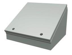
Saginaw operator consolet, NEMA 3R/4/12/13, 16 x 16 x 11in (HxWxD), desktop or pedestal mount, carbon steel, ANSI 61 gray, powder coat finish, single-door, 1/4-turn semi-flush latch.
