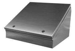
Saginaw operator consolet, NEMA 3R/4/4X/12/13, 16 x 16 x 11in (HxWxD), desktop or pedestal mount, 304 stainless steel, #4 brush finish, single-door, 1/4-turn semi-flush latch.
