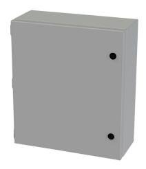
Saginaw Enviroline Junction series enclosure, NEMA 3R/4/12/13,  $16 \times 14 \times 6$  in (HxWxD), wall mount, carbon steel, ANSI 61 gray, powder coat finish, single-door, 1/4-turn semi-flush latch.
