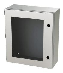
Saginaw Enviroline Junction series enclosure, NEMA 3R/4/4X/12/13,  $16 \times 14 \times 6$  in (HxWxD), wall mount, 316L stainless steel, #4 brush finish, single-door, 1/4-turn semi-flush latch, polycarbonate window.
