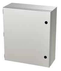
Saginaw Enviroline Junction series enclosure, NEMA 3R/4/4X/12/13, 16 x 14 x 6in (HxWxD), wall mount, 316L stainless steel, #4 brush finish, single-door, 1/4-turn semi-flush latch.
