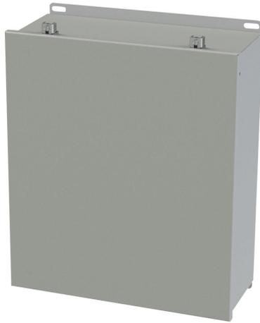
Saginaw enclosure, NEMA 3R/4/12/13, 14 x 16 x 6in (HxWxD), wall mount, carbon steel, ANSI 61 gray, powder coat finish, single-door, stainless steel clamps.
