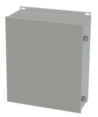
Saginaw enclosure, NEMA 3R/4/12/13,  $16 \times 14 \times 6in$  (HxWxD), wall mount, carbon steel, ANSI 61 gray, powder coat finish, single-door, stainless steel clamps.
