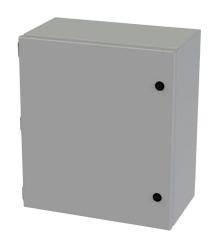
Saginaw Enviroline Junction series enclosure, NEMA 3R/4/12/13, 16 x 14 x 8in (HxWxD), wall mount, carbon steel, ANSI 61 gray, powder coat finish, single-door, 1/4-turn semi-flush latch.
