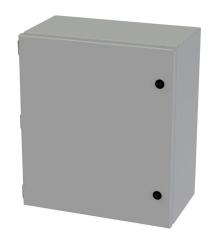
Saginaw Enviroline Junction series enclosure, NEMA 3R/4/12/13, 16 x 14 x 8in (HxWxD), wall mount, carbon steel, ANSI 61 gray, powder coat finish, single-door, 1/4-turn semi-flush latch.
