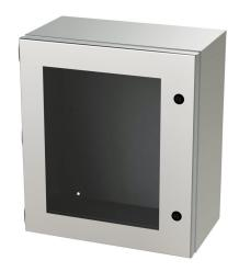
Saginaw Enviroline Junction series enclosure, NEMA 3R/4/4X/12/13,  $16 \times 14 \times 8$  in (HxWxD), wall mount, 304 stainless steel, #4 brush finish, single-door, 1/4-turn semi-flush latch, polycarbonate window.
