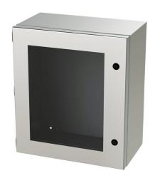
Saginaw Enviroline Junction series enclosure, NEMA 3R/4/4X/12/13, 16 x 14 x 8in (HxWxD), wall mount, 304 stainless steel, #4 brush finish, single-door, 1/4-turn semi-flush latch, polycarbonate window.
