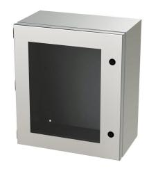
Saginaw Enviroline Junction series enclosure, NEMA 3R/4/4X/12/13,  $16 \times 14 \times 8in$  (HxWxD), wall mount, 316L stainless steel, #4 brush finish, single-door, 1/4-turn semi-flush latch, polycarbonate window.
