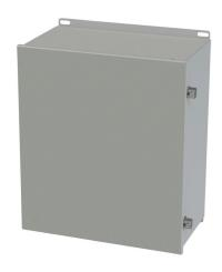
Saginaw enclosure, NEMA 3R/4/12/13, 16 x 14 x 8in (HxWxD), wall mount, carbon steel, ANSI 61 gray, powder coat finish, single-door, stainless steel clamps.
