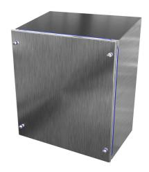
Saginaw sanitary enclosure, slope top, NEMA 3R/4/4X/12, 15 x 14 x 8in (HxWxD), wall mount, 304 stainless steel, #4 brush finish, screw cover.
