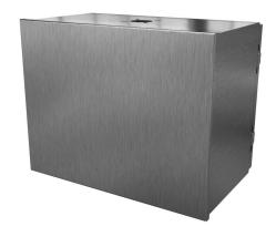
Saginaw HMI Enclosure, NEMA 3R/4/4X/12/13, 14 x 18 x 10in (HxWxD), suspension or pedestal mount, dual access, 304 stainless steel, #4 brush finish, screw cover front, single door rear, 1/4-turn semi-flush latch.
