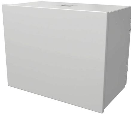
Saginaw HMI Enclosure, NEMA 3R/4/12/13, 14 x 18 x 10in (HxWxD), suspension or pedestal mount, dual access, carbon steel, RAL 7035 light gray, powder coat finish, screw cover front, single door rear, 1/4-turn semi-flush latch.
