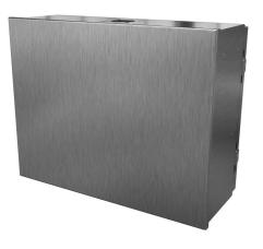
Saginaw HMI Enclosure, NEMA 3R/4/4X/12/13, 14 x 18 x 6in (HxWxD), suspension or pedestal mount, dual access, 304 stainless steel, #4 brush finish, screw cover front, single door rear, 1/4-turn semi-flush latch.
