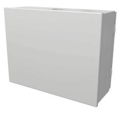
Saginaw HMI Enclosure, NEMA 3R/4/12/13, 14 x 18 x 6in (HxWxD), suspension or pedestal mount, dual access, carbon steel, RAL 7035 light gray, powder coat finish, screw cover front, single door rear, 1/4-turn semi-flush latch.
