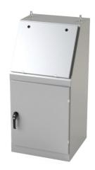
Saginaw operator console, NEMA 3R/12/13, 50 x 24 x 23in (HxWxD), freestanding, dual access, carbon steel, ANSI 61 gray, powder coat finish, single-door, 3-point keylocking/padlocking combo handle.
