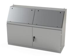
Saginaw operator console, NEMA 3R/12/13, 50 x 72 x 23in (HxWxD), freestanding, dual access, carbon steel, ANSI 61 gray, powder coat finish, double-door, 3-point keylocking/padlocking combo handle.
