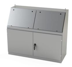
Saginaw operator console, NEMA 3R/12/13, 50 x 60 x 23in (HxWxD), freestanding, dual access, carbon steel, ANSI 61 gray, powder coat finish, double-door, 3-point keylocking/padlocking combo handle.
