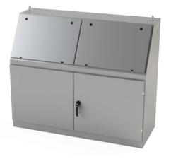
Saginaw operator console, NEMA 3R/12/13, 50 x 60 x 23in (HxWxD), freestanding, dual access, carbon steel, ANSI 61 gray, powder coat finish, double-door, 3-point keylocking/padlocking combo handle.
