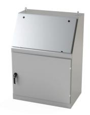
Saginaw operator console, NEMA 3R/12/13, 50 x 36 x 23in (HxWxD), freestanding, dual access, carbon steel, ANSI 61 gray, powder coat finish, single-door, 3-point keylocking/padlocking combo handle.
