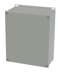
Saginaw enclosure, NEMA 3R/4/12/13, 14 x 12 x 6in (HxWxD), wall mount, carbon steel, ANSI 61 gray, powder coat finish, screw cover.
