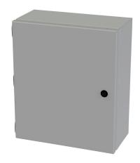
Saginaw Enviroline Junction series enclosure, NEMA 3R/4/12/13,  $14 \times 12 \times 6$  in (HxWxD), wall mount, carbon steel, ANSI 61 gray, powder coat finish, single-door, 1/4-turn semi-flush latch.
