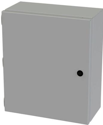
Saginaw Enviroline Junction series enclosure, NEMA 3R/4/12/13, 14 x 12 x 6in (HxWxD), wall mount, carbon steel, ANSI 61 gray, powder coat finish, single-door, 1/4-turn semi-flush latch.
