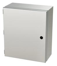
Saginaw Enviroline Junction series enclosure, NEMA 3R/4/4X/12/13,  $14 \times 12 \times 6in$  (HxWxD), wall mount, 304 stainless steel, #4 brush finish, single-door, 1/4-turn semi-flush latch.
