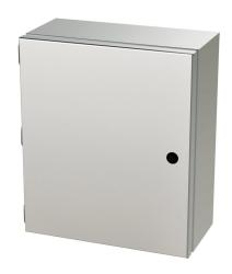
Saginaw Enviroline Junction series enclosure, NEMA 3R/4/4X/12/13, 14 x 12 x 6in (HxWxD), wall mount, 316L stainless steel, #4 brush finish, single-door, 1/4-turn semi-flush latch.
