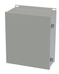
Saginaw enclosure, NEMA 3R/4/12/13, 14 x 12 x 6in (HxWxD), wall mount, carbon steel, ANSI 61 gray, powder coat finish, single-door, stainless steel clamps.
