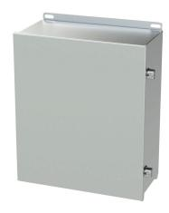
Saginaw enclosure, NEMA 3R/4/4X/12/13, 14 x 12 x 6in (HxWxD), wall mount, 304 stainless steel, #4 brush finish, single-door, stainless steel clamps.
