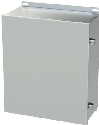
Saginaw enclosure, NEMA 3R/4/4X/12/13, 14 x 12 x 6in (HxWxD), wall mount, 316L stainless steel, #4 brush finish, single-door, stainless steel clamps.
