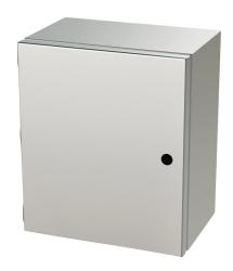
Saginaw Enviroline Junction series enclosure, NEMA 3R/4/4X/12/13, 14 x 12 x 8in (HxWxD), wall mount, 304 stainless steel, #4 brush finish, single-door, 1/4-turn semi-flush latch.
