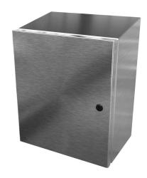
Saginaw Enviroline Junction series enclosure, slope top, NEMA 3R/4/4X/12/13,  $14 \times 12 \times 8$  in (HxWxD), wall mount, 304 stainless steel, #4 brush finish, single-door, 1/4-turn semi-flush latch.
