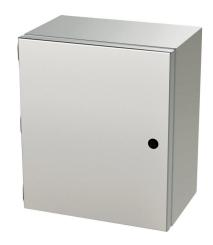
Saginaw Enviroline Junction series enclosure, NEMA 3R/4/4X/12/13, 14 x 12 x 8in (HxWxD), wall mount, 316L stainless steel, #4 brush finish, single-door, 1/4-turn semi-flush latch.
