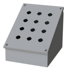
Saginaw pushbutton consolet, 12 holes, 22mm, NEMA 4/12/13, 11 x 9 x 9in (HxWxD), wall mount, carbon steel, ANSI 61 gray, powder coat finish, screw cover, purchase subpanel separately.
