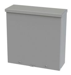
Saginaw enclosure, NEMA 3R, 12 x 12 x 4in (HxWxD), wall mount, carbon steel, ANSI 61 gray, powder coat finish, screw cover, padlock hasp and staple.
