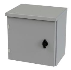
Saginaw enclosure, NEMA 3R, 12 x 12 x 8in (HxWxD), wall mount, carbon steel, ANSI 61 gray, powder coat finish, single-door, 1/4-turn padlocking wing handle.
