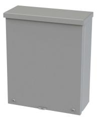
Saginaw enclosure, NEMA 3R,  $12 \times 10 \times 4$ in (HxWxD), wall mount, carbon steel, ANSI 61 gray, powder coat finish, screw cover, padlock hasp and staple.
